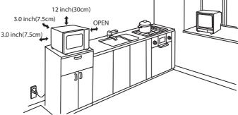
A minimum clearance of 3.0 inches (7.5cm) is required between the oven and any adjacent walls. One side must be open.
