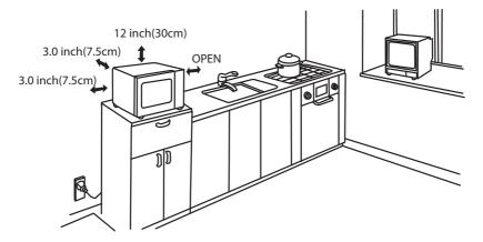
A minimum clearance of 3.0 inches (7.5cm) is required between the oven and any adjacent walls. One side must be open.
